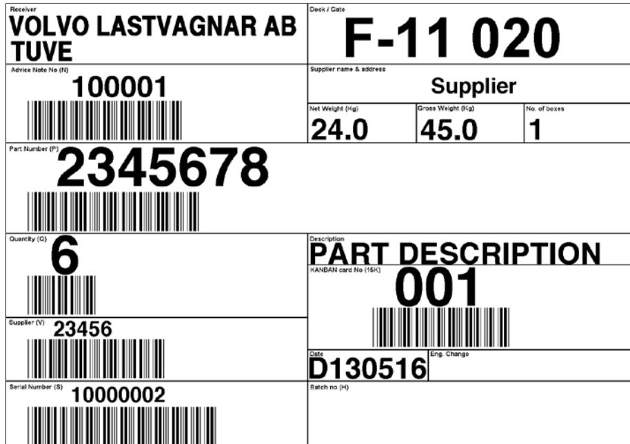
9 Kanban Simplified Handling Unit (S) Label attached to the pallet.
